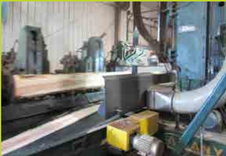
⤴ Sawdust suction in the head throat at Tusco. Image Credit: Conrad Bates
