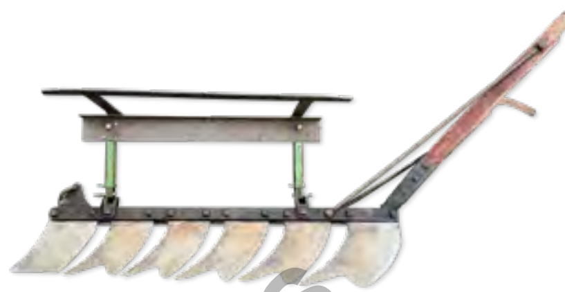
A blade that is pulled by a horse (during the ice harvest).
